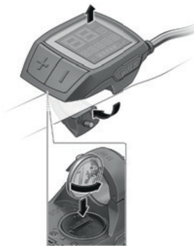
Image 30: Changing the batteries of the Purion display
