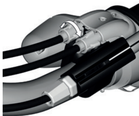
Image 41: Reducing or increasing cable slack by turning the barrel at the grip shifter
