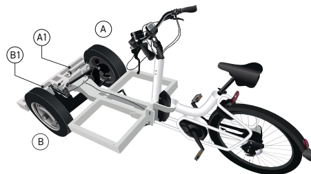
Image 32: Removing and placing a front tyre
