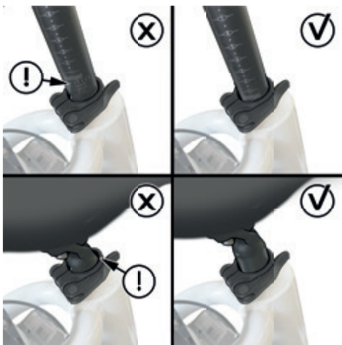
Image 7: Max and min insertion seat post
