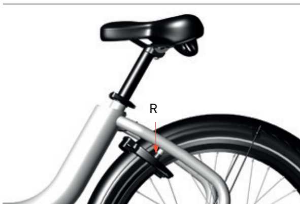
Image 38: Checking the lock rubbers
