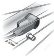
Image 31: Distance between the speed sensor and the speed sensor magnet
