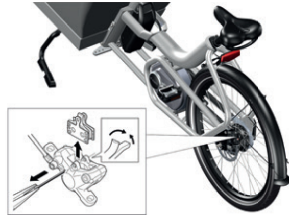
Image 39: Removing the brake pads in order to check them for wear
