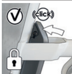
Image 18: Feedback correctly fitted battery
