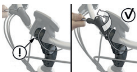
Image 9: Loosening the bolt on the stem
