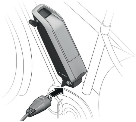
Image 29: Plugging charger plug in charge socket on the bottom part of the battery holder
