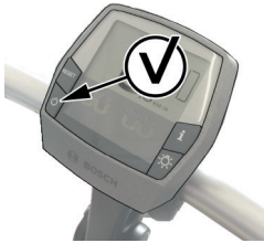
Image 21: Switching the display on and off
